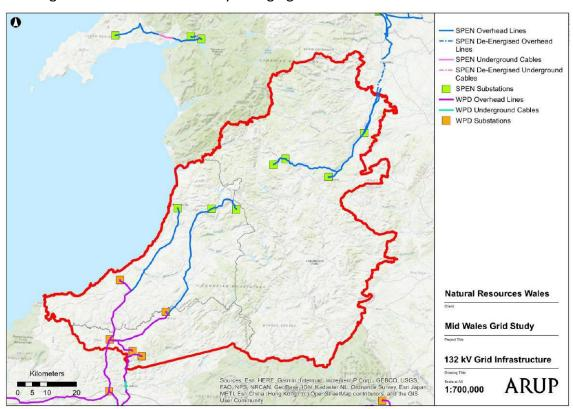
Our proposals for Mid-Wales accommodate forecast additional demand through to the early 2030s. However, a collaborative Whole Systems planning approach is required to identify the optimal longer-term distribution and transmission solution to upgrade the Mid-Wales network to
